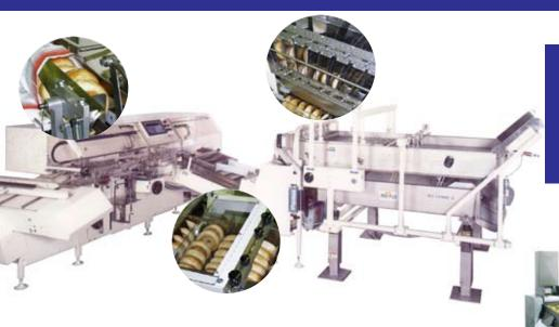
The Formost Bagel System features highly efficient aligning mechanism for bagging bagels. Feed mechanism consists of a shaker table, laning guides, drop chute, and rotary indexer. The unit deposits counted and stacked bagels into a Formost bagger bucket infeed conveyor.
