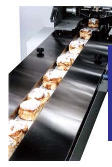
Attachless Infeed Conveyor automatically indexes soft and sticky products into a Fuji-Formost horizontal wrapper at speeds up to 120 packages per minute. Computer controlled flat belts have no lugs and are easy to remove and clean.
