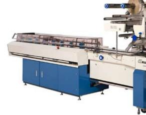
The Fuji-Formost FFS-1000 High Speed Infeed has a multiple belt conveyor system with automatic control of each belt according to product delivery. Shown below with Formost product alignment system. Complete system with Formost Transpositor on front cover.
