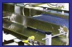
After the product is placed in the bag, the bag openers release and product motion separates the bag from the wicket.
