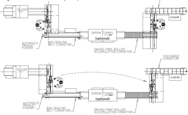
The inner bag is sealed creating a tight, attractive and tamper evident package. The bag can be run through a shrink tunnel for an even tighter package.
